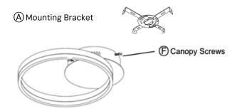
Twist canopy to lock fixture in place. Secure canopy with canopy screws (F).
