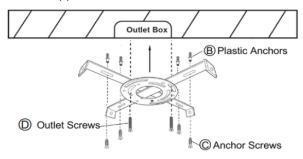
Attach included mounting bracket (A) to outlet box with outlet screws (D). Screw anchor screws (C) into plastic anchors (B) to secure mounting bracket (A).
